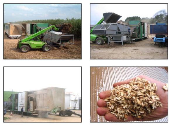
Pictures 5 (Clockwise): Front loader loading billets into chipper, conveyor belt feeds billets into chipper, modified plastics chipping unit, very fine quality wood chip
